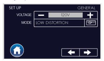
Voltage Regulation: The Power Plant 5 provides user adjustment of the output voltage. By applying touch to either the "+" or "-" selector, one can adjust the output voltage by one-volt increments.
