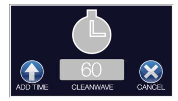
By selecting the icon labeled CLEAN the Power Plant 5 will activate the CleanWave function and the display of the P5 will begin to countdown the time left as the P5 is applying the CleanWave signal. CleanWave places a series of higher frequencies that ride on the main sine wave to help "degauss" connected magnetics. To ensure that CleanWave is effective, make sure all connected equipment is on and functioning. CleanWave can be used between CD's, movies and vinyl. It is not recommended
