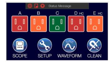
exhibiting green receptacle icons and will remain at the HOME SCREEN. The illuminated front-panel display is touch-activated. By touching any of the output receptacle icons, one can toggle that zone on & off. Upon turning off, the output receptacle icon will turn red. Below these output receptacle icons one will find selector icons for Scope, Setup, Waveform, and Clean.
